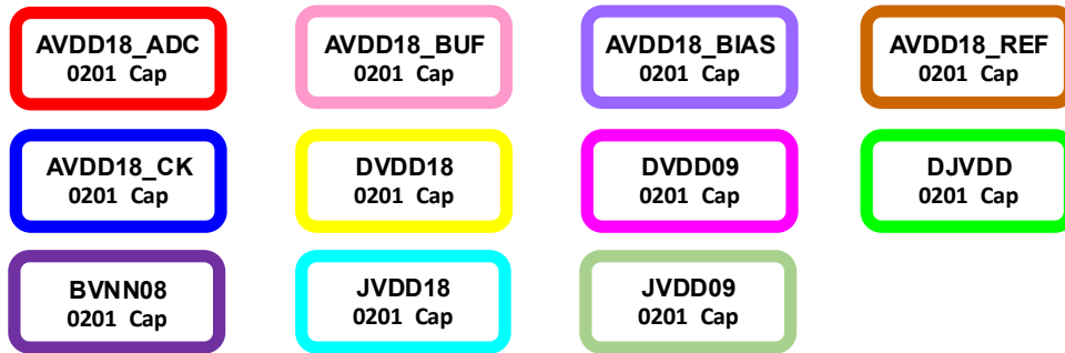
Fig 8-14. Recommend Decoupling Capacitor Placement on Power Supplies
